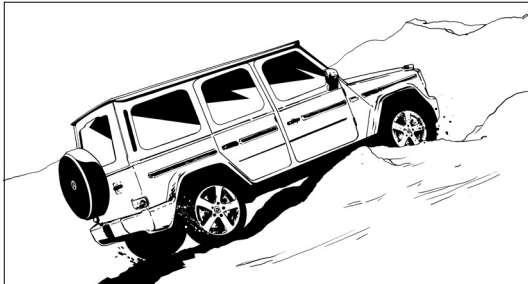
Large ramp breakover angle:
